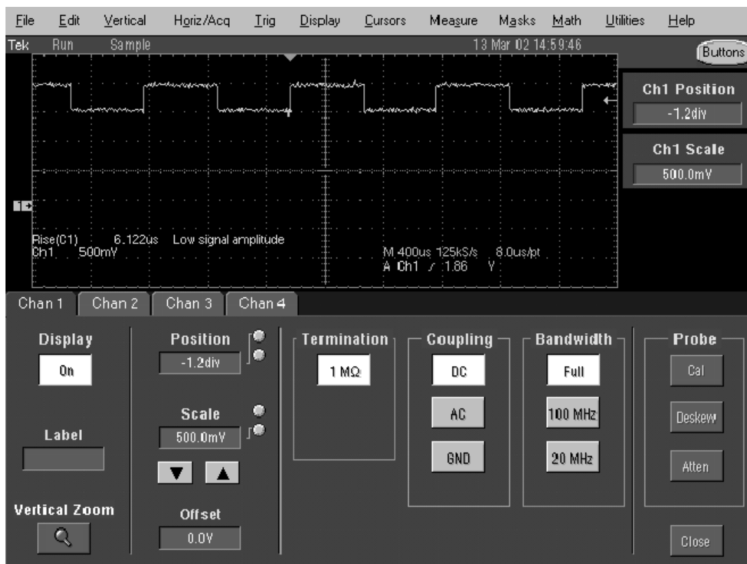
Figure 12: Typical waveform at DC Coupling
